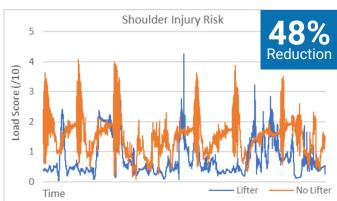
The above charts demonstrate the correct use of the vacuum lifter reduced the load on the worker's back by 32% and shoulder by 48%.
